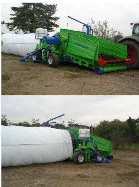
Figure 1 and 2. Press for filling polyethylene films with fresh biomass
