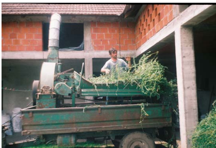
Figure 1. Ensiling of alfalfa biomass using silo-shredder (Globoder)
