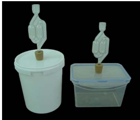
Figure 1. Non-transparent (Čolović et al. , 2010) and transparent mini-silo
